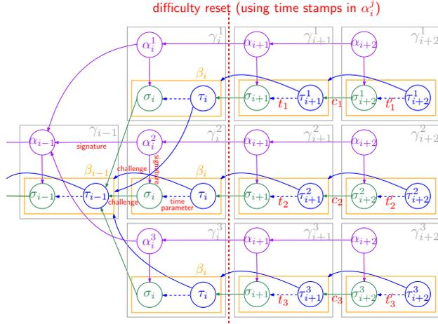
Figure 7: Illustration of the grinding attack on the difficulty parameter discussed in §5.2, where slightly different timestamps in the foliage blocks  $\alpha_i^1, \alpha_i^2, \alpha_i^3$  right before the difficulty reset at depth  $i$  lead to different PoSpace challenges  $c_1, c_2, c_3$  for the blocks at depth  $i + 2$ .
