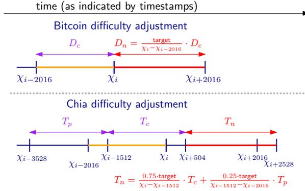
Figure 8: Illustration of the difficulty adjustment in Bitcoin and Chia. In Bitcoin the difficulty for the new epoch  $D_n$  (in red) is computed using the timestamps of the epoch  $D_c$  right before it (in orange). In Chia the period to compute the new difficulty  $T_n$  is shifted one fourth of an epoch backwards.
